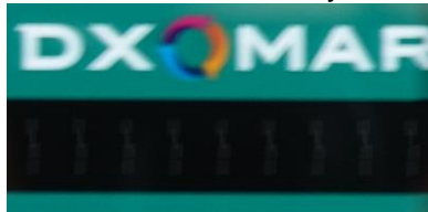
Figure 60 Illustration picture of the motion blur test pattern
