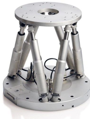
Figure 2. Hexapod PI M-840 motion platform used for our evaluation. The six axes are driven by a specific controller to set the position and the orientation of the platform.
