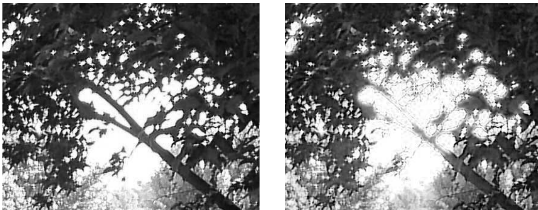
Figure 1. Digital photograph of a backlit tree. Left: luminance channel. Right: blue channel. The blue channel exhibits obviously too large values inside the branches. Since the other channels are dark (as they should be), the branches show large color fringes. The width of these fringes can be at least 4 or 5 pixels.
