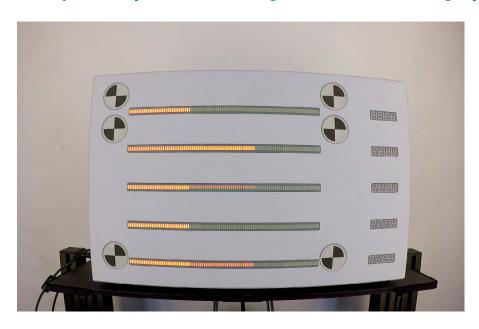
ANALYZER's automatic flicker measurement is compatible with wide-angle cameras and can handle highly distorted images, ensuring good accuracy for any field of view up to 170°.
