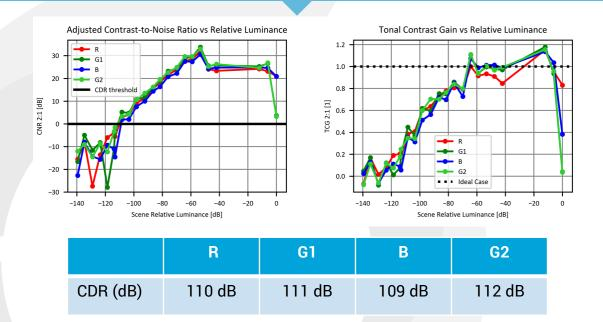
The P2020 dynamic range (CDR) value is only 10dB lower than the sensor level dynamic range, which means that the lens is well fitted to the sensor.
