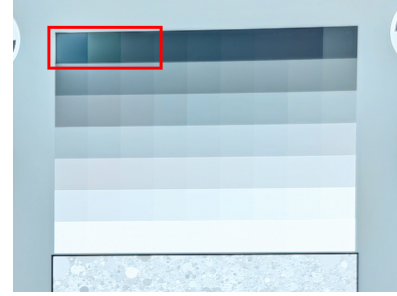
Figure 6. Example of tone inversion: the patch that is darker in the real scene appears brighter in the picture (likely because of the interaction of lens glare and local tone-mapping algorithms).
