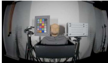
Lab test example: setup used for Texture, Color, Exposure and Timing measurements.
