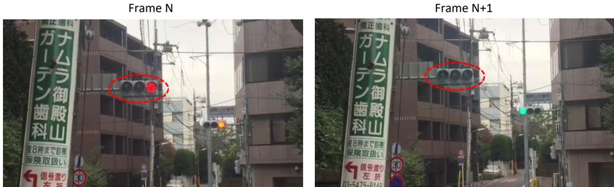
NOTE—The images above show two consecutive frames from a video sequence. In frame N, the traffic light in the front (highlighted in red dashed circle) appears with red light on. However, in frame N+1, the traffic light in the front, which is still visually observed by a human as a red light on, is no longer captured by the camera, thus leading all lights of the traffic light to appear off.
