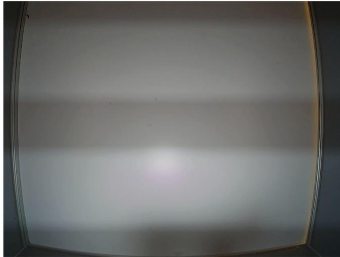
NOTE—This image was captured with a rolling shutter image sensor. In this example, the scene is illuminated by a diffuse LED light source, driven by a 75Hz, 10% duty cycle signal. The image shows a typical banding effect with darker horizontal stripes, representing the rows missing the exposure of LED illumination ON timing.
