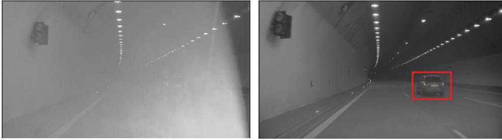
NOTE—Two sequential video frames while entering a tunnel that demonstrate contrast reduction by veiling glare, caused by sunlight illuminated dust particles. In the left image, the effect significantly hinders the recognition of a preceding car while in the right image (only a few milliseconds later) the sunlight is blocked away and a robust detection of the car is possible.
