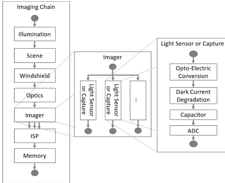
**Figure 11 Example flow diagram of an imaging chain<sup>6</sup>**
