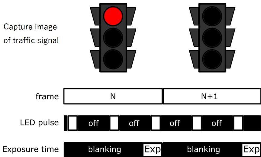
NOTE—In frame N, the LED pulse and the camera exposure time coincide, and the traffic light is captured. In frame N+1, the LED pulse and exposure time do not coincide, and the traffic light appears off.
